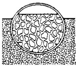
Spaces between particles leave untreated concrete subject to penetration by moisture, oils, acids, etc.
