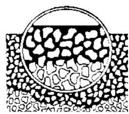
CONSEAL penetrates into the concrete where it reacts with free lime and alkali to fill the voids and bond the particles into a solid mass, creating a permanent seal.
